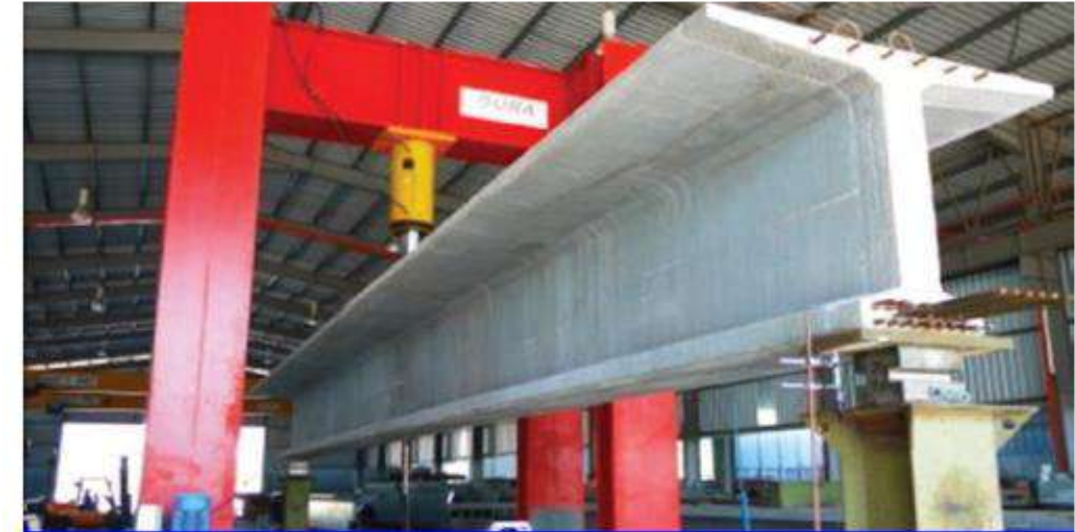
Flexural Strength Verification Test Set-up
