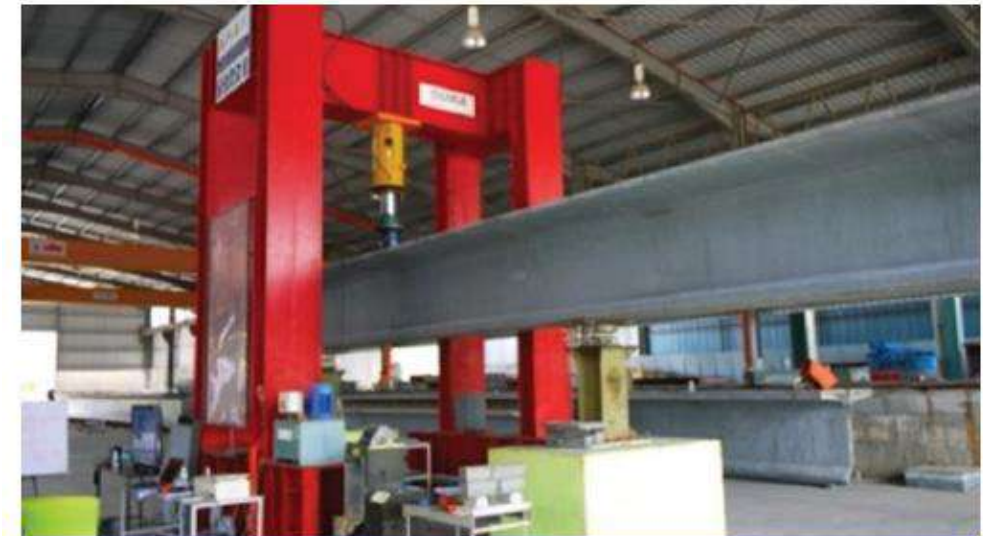
Shear Strength Verification Test Set-up
