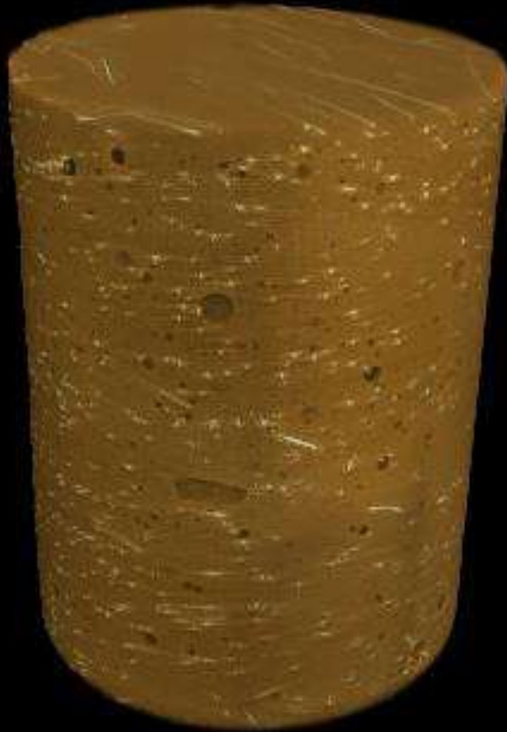
CT Scan on core sample
